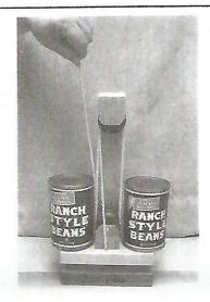
1. In Step 2, there was less force required to lift the weight using the block and tackle. In principle, what reduction in force is possible using this device? (In fact, as noted, it should be 1/5, but it will be more than this.)
