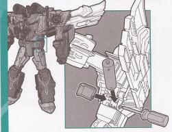
TO REPLACE BATTERY 1x 1.5V AA ALKALINE BATTERY Replace demo battery with alkaline battery. Use a Phillips/cross head screwdriver (not included).
